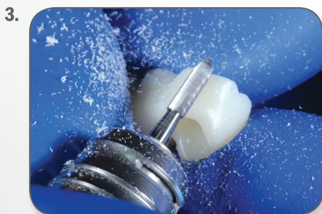
The H139PSQ.023 PMMA Cutter is used to reduce sprues and contour provisional without clogging of the instrument.
