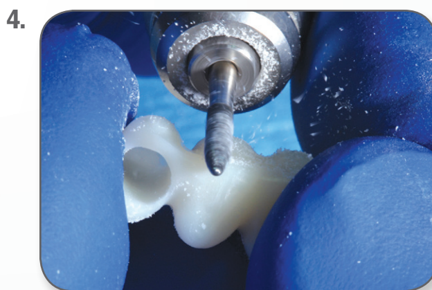
PMMA Cutters can be utilized to trim and contour any other surface of the restoration. Recommended speed is 15,000 rpm.
