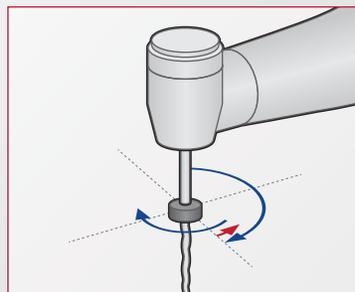
**Traditional Reciprocation** file systems can only reciprocate back and forth without any regard for torque resistance. Torque is unmonitored in a pure reciprocation handpiece.
