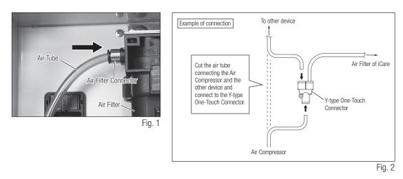
• The optimum air pressure for this product is between 0.5 - 0.6MPa (5 - 6kgf/cm<sup>2</sup>). The product does not operate if the air pressure is set less than 0.5MPa (5kgf/cm<sup>2</sup>).
